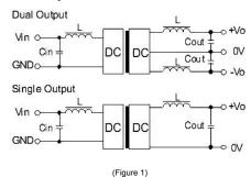
It should also be noted that the inductance and the frequency of the "LC" filtering network should be staggered with the DC/DC frequency to avoid mutual interference. However, the capacitance of the output filter capacitor must be proper. If the capacitance is too big, a startup problem might arise. For every channel of output, provided the safe and reliable operation is ensured, the greatest capacitance of its filter capacitor sees (Table 1).
